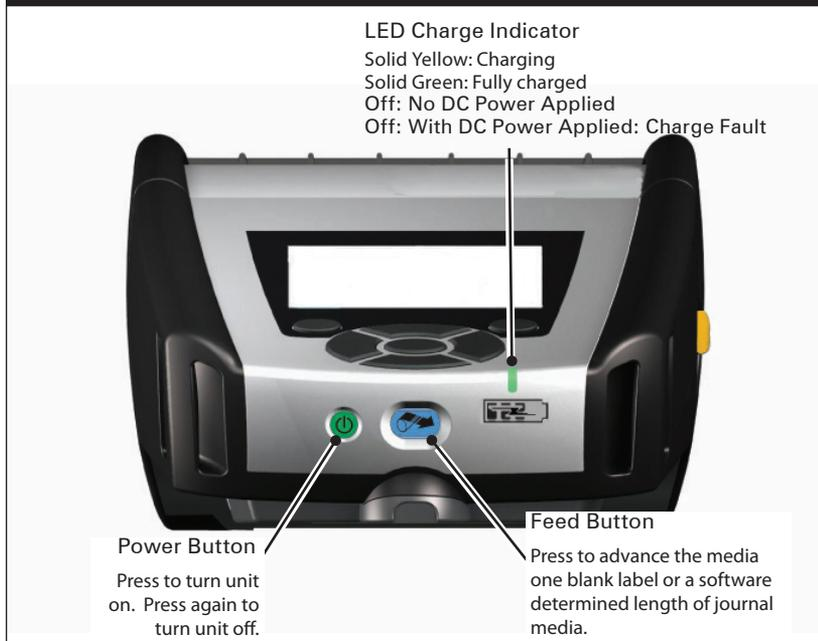
Figure 17a: Standard Control Panel (QLn420)
